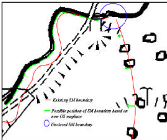
Fig. 1. An illustration of an unclosed SM polygon and problems associated with changes in the OS map base.
